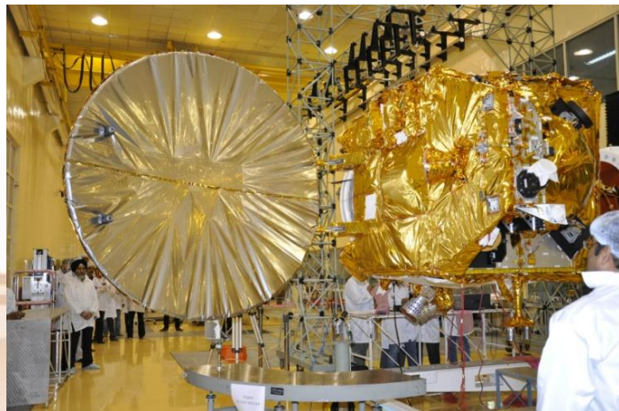
Antenna Deployment Test
