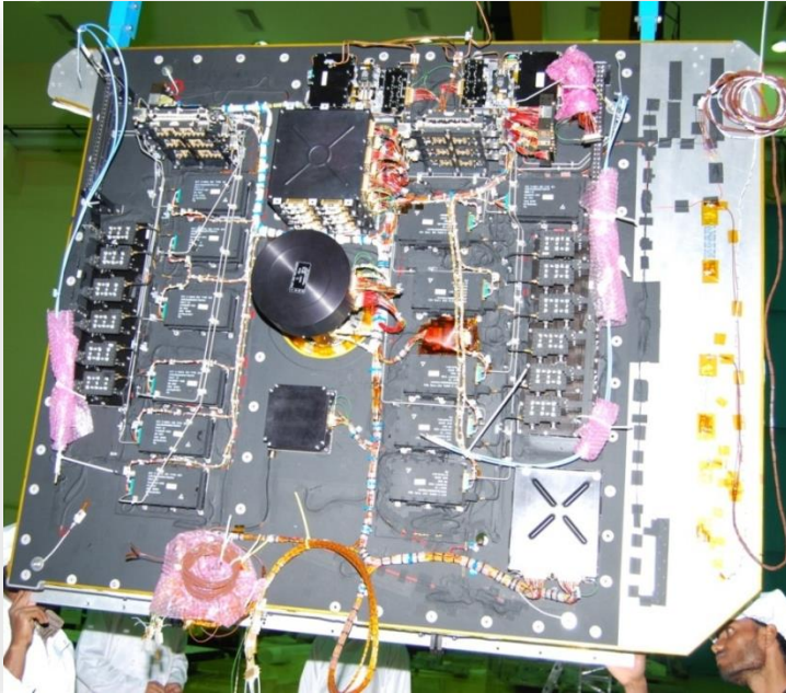
SOUTH PANEL READY FOR ASSEMBLY
