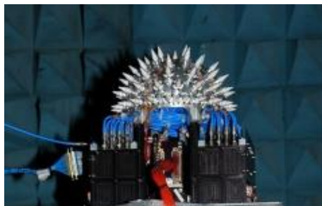
Phased array antenna
