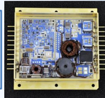
30W HMC DC-DC CONVERTER (+15V: 500mA, -15V: 500mA, +5V: 3A)
