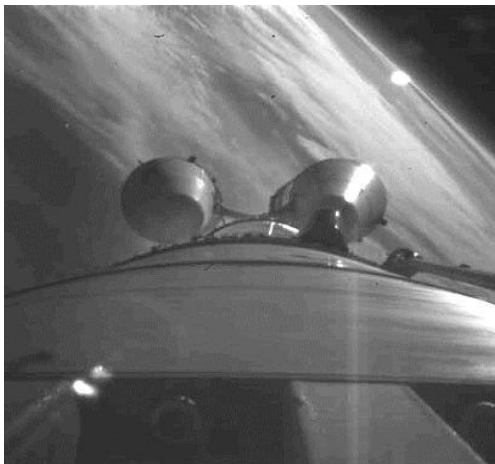
Video Imaging camera on Launch Vehicle
