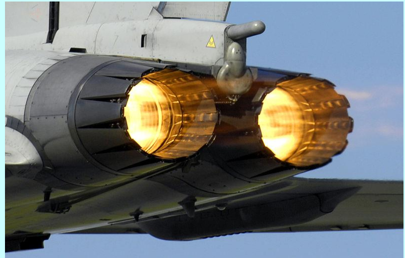
Rear mounted IR sensor ( above aircraft engine)
