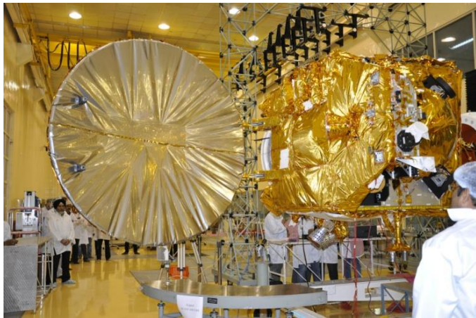
HGA-Antenna Deployment Test
