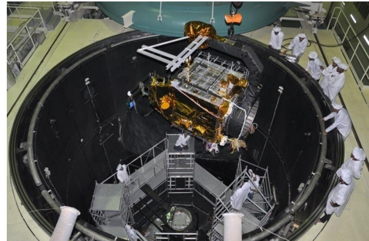
Loading into Thermovac Chamber
