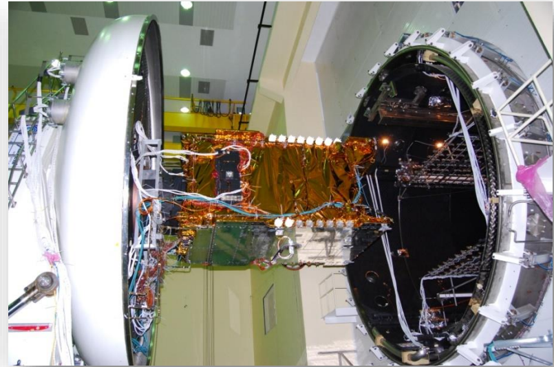
Loading to Thermovac Chamber
