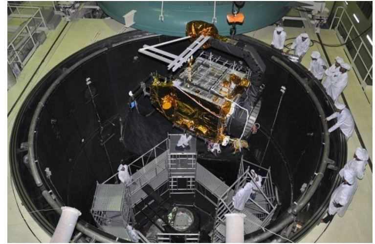
Loading to Thermovac Chamber Aug 2013
