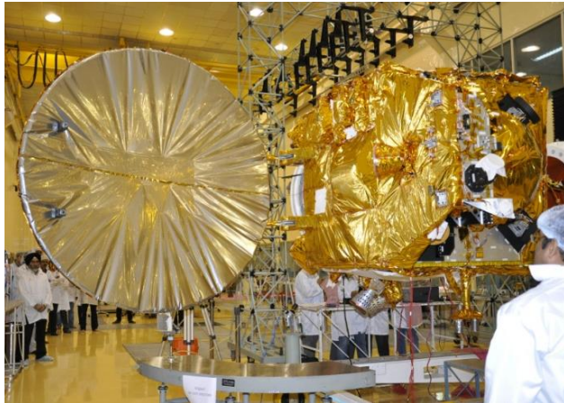
Antenna Deployment Test Sep 2013
